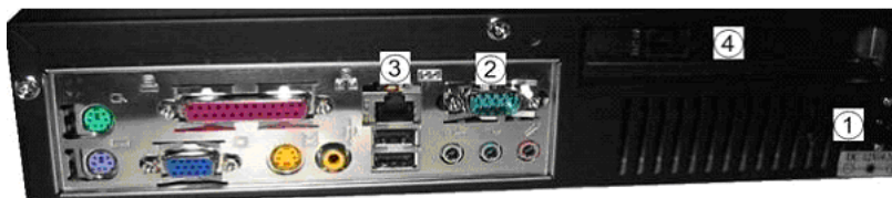
Fig 1.2: Interfaces on the rear side of the HomeServer.
