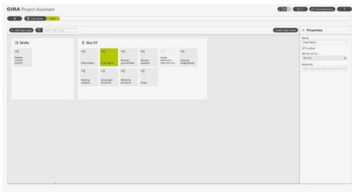
5. Processing logic pages: The GPA features a simple graphic editor for creating logic pages. Numerous logic pages can be used, switched to active or inactive, as well as structured and quickly relocated using tags.
